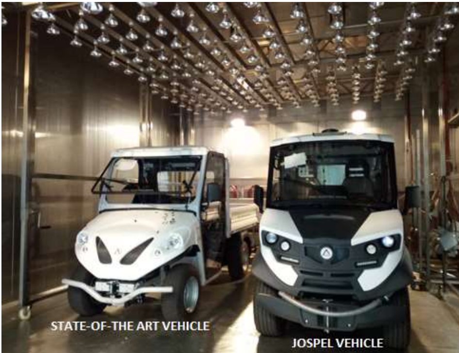
Climatic chamber to evaluate thermal comfort
